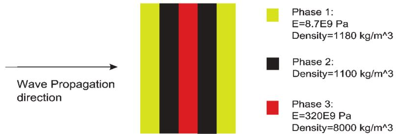
FIG. 2. Schematic of a 3-phase unit cell.
